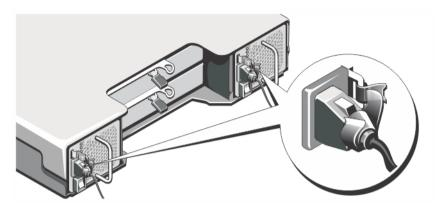
Figure 3. Securing the Power Cable(s)
